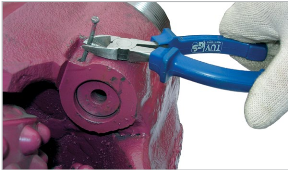
1. Remove the nail to remove the nozzle
