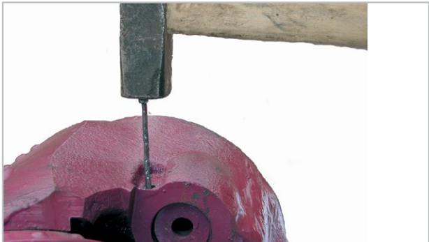
4. Fix the nozzle with a nail using a hammer
